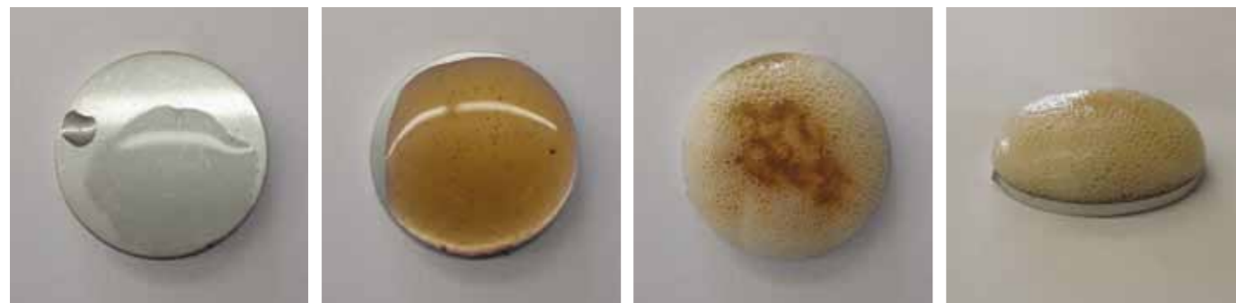
1. Stainless steel surface moistened with water. 2. Negative reaction after using BioFinder on a non contaminated surface. 3. Positive reaction after using BioFinder on a surface contaminated with biofilms. 3b. Side view of a positive reaction after using BioFinder on a surface contaminated with biofilms.
